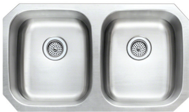
SIN-18-DBLBWL-5050-3118 Outside - 32 1 / 4 " x 18 1 / 2 " Left Inside - 14 1 / 2 " x 16 1 / 2 " Right Inside - 14 1 / 2 " x 16 1 / 2 " Depth - 8" Minimum Cabinet - 36" 1 Strainer included Matching Grid Available
