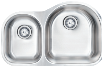
SIN-18-DBLBWL-4060-3120 Outside - 30 3 / 4 " x 19 1 / 2 " Left Inside - 11" x 14 1 / 2 " Right Inside - 16 1 / 2 " x 17 1 / 2 " Depth - 7 1 / 2 " / 9" Minimum Cabinet - 36" 1 Strainer included Matching Grid Available
